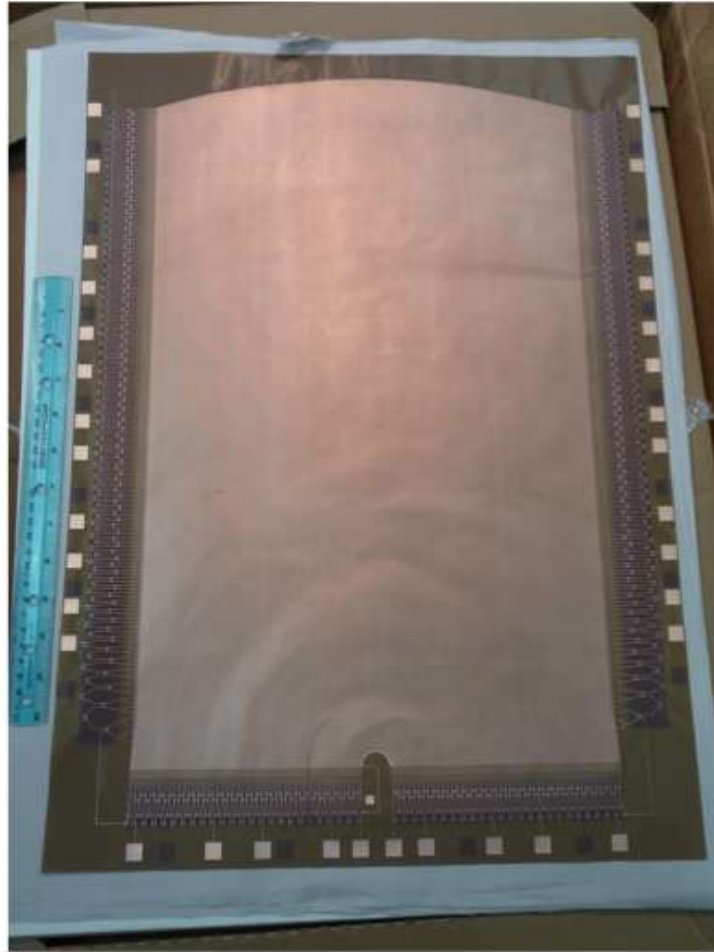
Figure 3.11: Photograph of a large rf carpet with a 48 cm transport distance and a pitch of 0.38 mm. The collection electrode (center bottom of the transport area) has a diameter of 1.8 cm.
